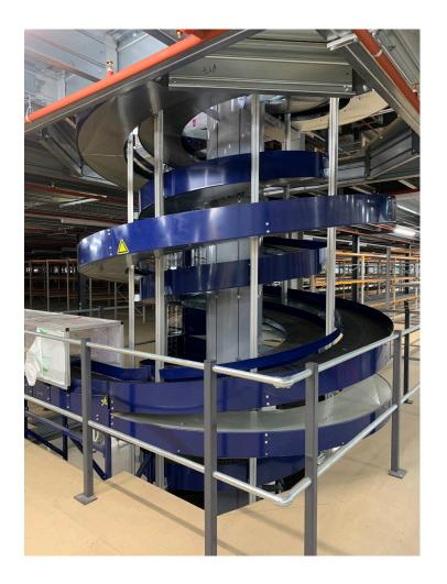
On the ground floor a recirculating carousel system feeds the filled tote bins to a series of packing lanes. Prioritisation of the tote order to a designated lane, where the contents are removed and packed, provides the Gardiners operational team with a fully flexible automated packing solution. Empty tote bins are re-designated and returned onto the recirculating system ready for the fulfilment of new orders.
